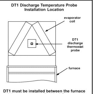
and the evaporator coil with airflow arrow in correct position. Upflow application shown.
